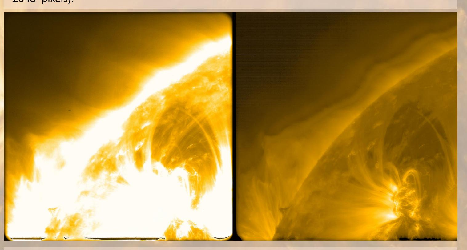
Left: high-gain only HRI-EUV image, showing large parts of the Sun over-exposed, but good signal in the fainter parts of the images. The dark lines at the bottom are detector artifacts and are in fact showing some low-gain pixels. Right: low-gain only HRI-EUV image. There are no longer over-exposed pixels, but the image shows several ringing artifacts in darker areas of the image.
